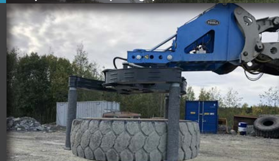
35° or 90° tilt module - horizontal to vertical
