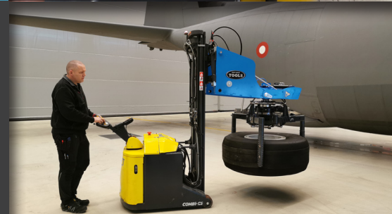
90° tilt and precise +/-25° rotation
